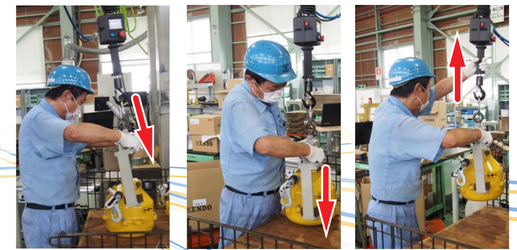
Manual operation sets the jig smoothly
